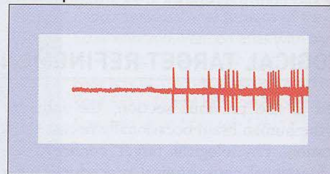
Figure 52.31 Microelectrode recording trace beginning in the relatively acellular zona incerta. Note the larger background noise indicated by the thicker baseline upon entry into the more cellular subthalamic nucleus.
