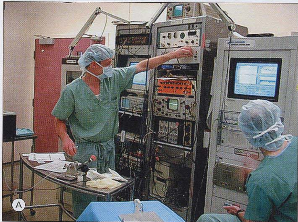
Figure 52.29 (A) Microelectrode recording amplifiers, recorders, and displays in a full rack configuration. (B) Compact laptop-based microelectrode recording system sitting atop a microstimulator unit (green arrow).
